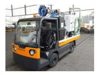
The **NEU Toilet Servicing Mobile Unit** is a hygienic way to empty toilet retention tanks on rail vehicles. A vacuum pump sucks the effluent into a depressurized tank on the mobile unit. If required, the toilet tanks are then rinsed with a clean water spraying nozzle. If rinsing is required, the rinsing water is also sucked into the mobile unit tank. The tank is pressurized to discharge the collected effluent into a collector tank, a recycling station or direct to the sewer.
